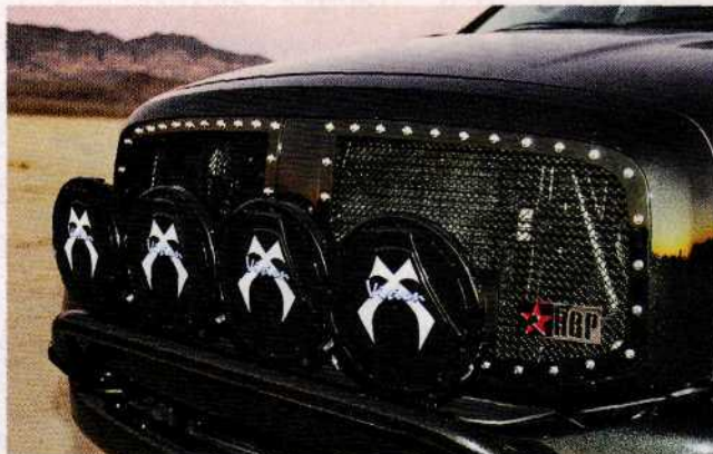
Adding style to the outside of the Megacab is a grille from RBP protected by a light bar that houses four Vision X HID auxiliary lights. The snout of the Dodge was also shod with headlights from an SRT-10 and the front bumper was color-matched.
