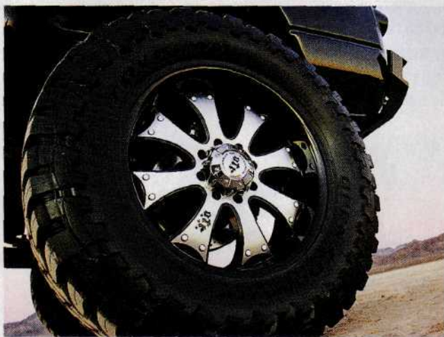
I.C.C.E. OTR wheels measuring 20 inches in diameter and 11 inches in width are surrounded by 40x15.5 Toyo Open Country MT tires and upgraded brakes from SSBC are used in the front and rear.
