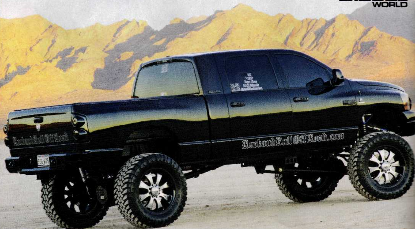
I.C.C.E. OTR wheels measuring 20 inches in diameter and 11 inches in width are surrounded by 40x15.5 Toyo Open Country MT tires and upgraded brakes from SSBC are used in the front and rear.
